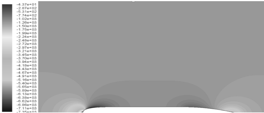
Figure 4: Contours of pressure around bare submarine hull DREA (filled)
