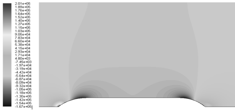
Figure 10: Contour of pressure around the surface of AUV ( L/D=6 )
